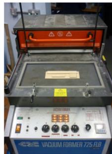
1. Place the mould on the bed of the machine.
