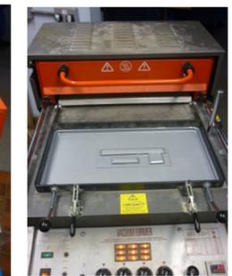
5. Raise the mould, turn on the vacuum pump.
